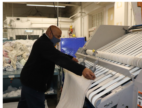
Almost all linen that goes through the facility is machine folded, except for pajamas and washcloths, which are folded by hand.
